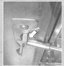
Undo the screw using a 7mm socket wrench and remove the door catch.
