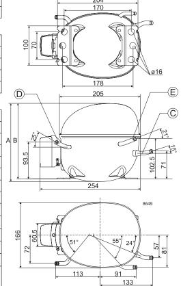
**EN 12900 Household (CECOMAF)** 220V, 50Hz, RC 4 μF, ePTC consumption incl., static cooling
